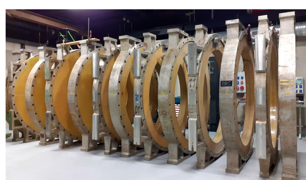
Picture showing the 13 copper coils after their installation in SPEKTRE experimental room.
