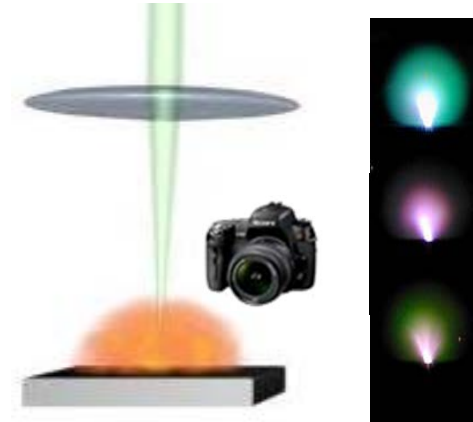
Solid target (ablation) Application: film deposition, analysis...
